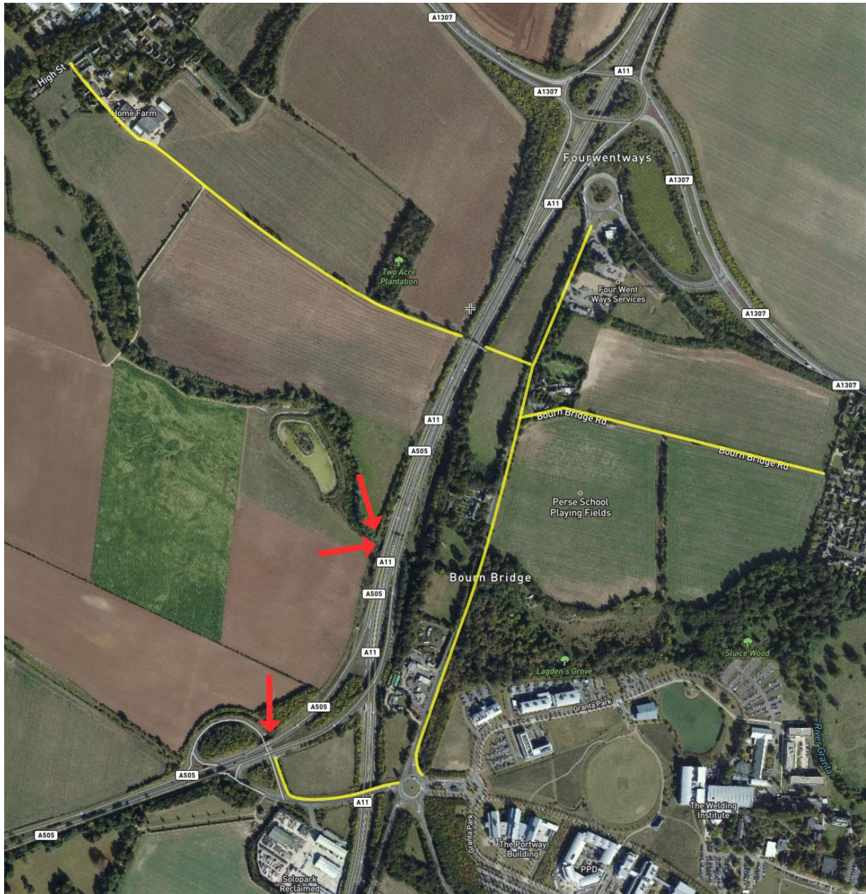
Figure 10: Cycle routes between Babraham and Granta Park and Abingtons in need of upgrading. Red arrows indicate possible new A11/A505 crossing points (north or south bank of River Granta or alongside A505 slip ramp)
